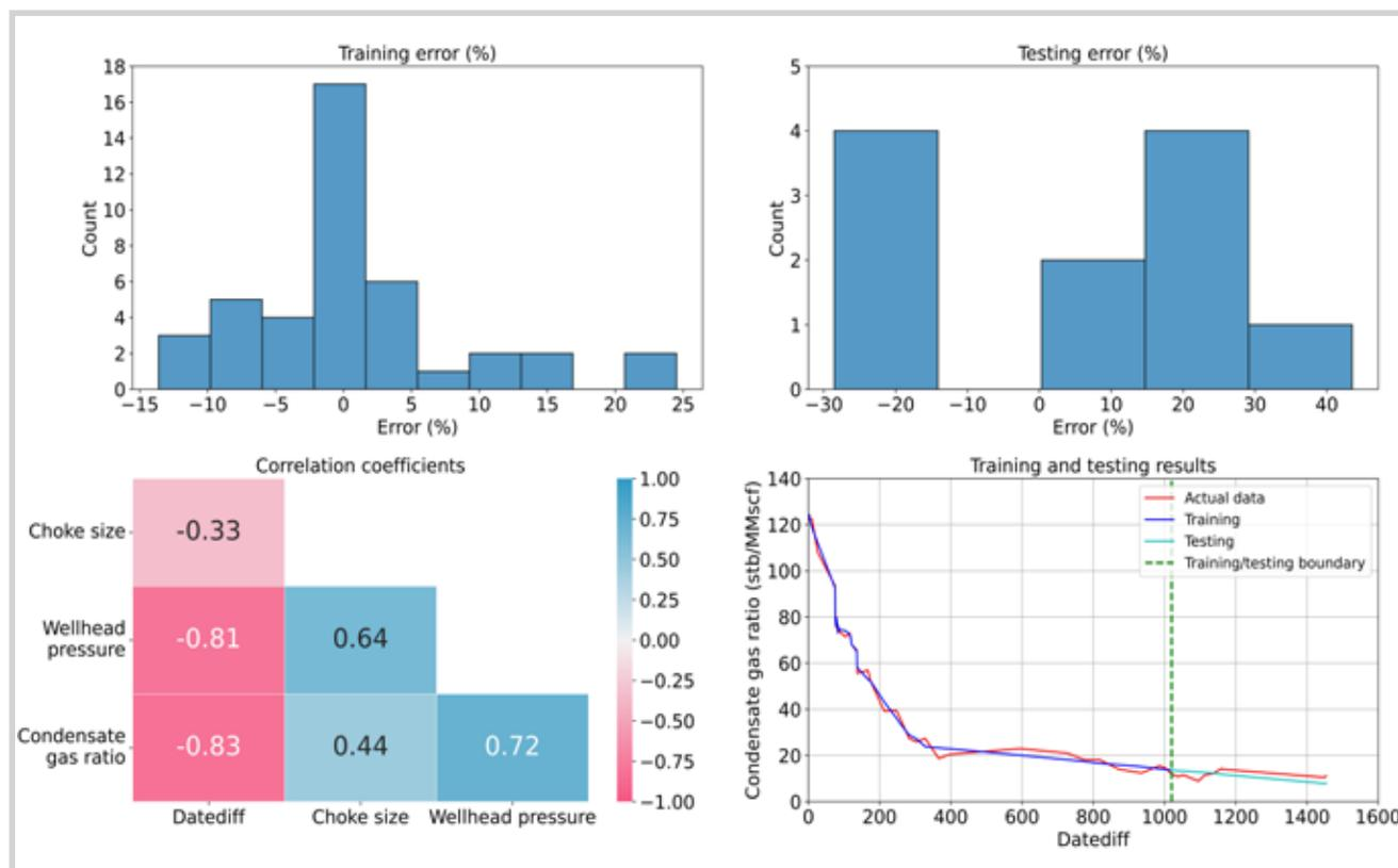
Figure 7. HT-X CGR prediction using piecewise regression and linear regression with split ratio of training and testing dataset of 80/20.
